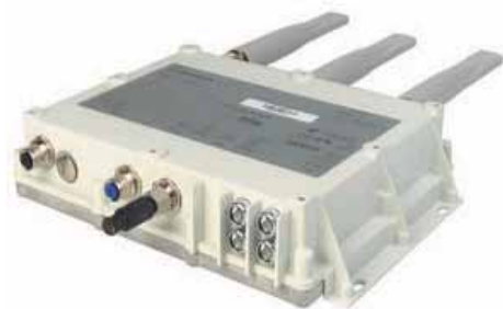
Figure 8: Connectors for external antennas on TCSNWA271 and TCSNWA2A1
