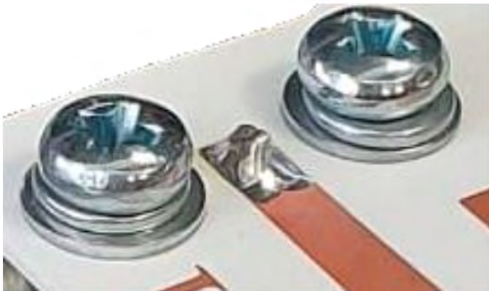
Because pins are soldered at both ends, the whole connection is monolith and permanent, antenna can't be detached without desoldering.
