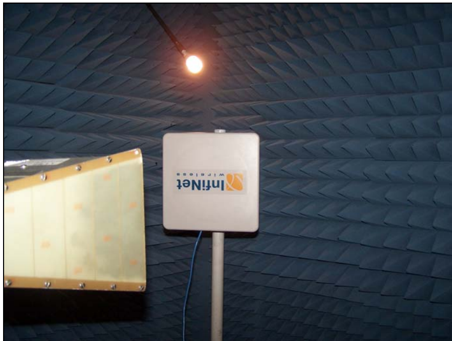
Photograph 2. Radiated Spurious Emissions, Above 1 GHz, Test Setup
