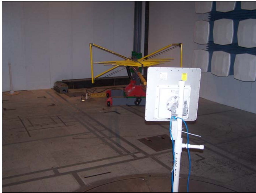
Photograph 1. Radiated Spurious Emissions, Below 1 GHz, Test Setup
