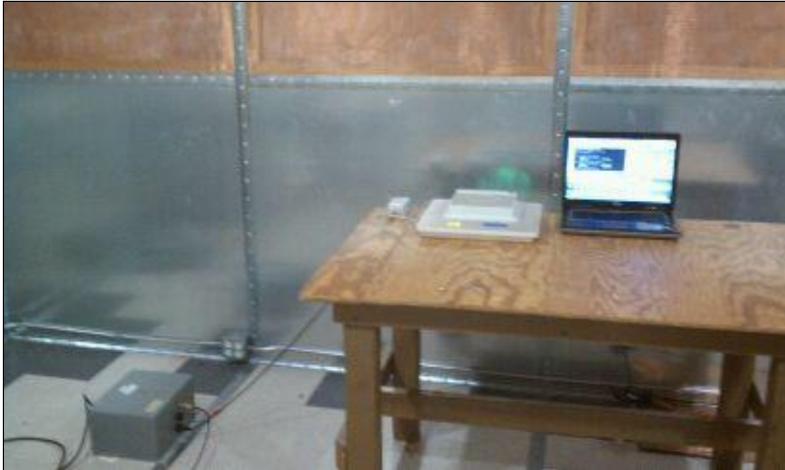
Photograph 4. Conducted Emissions, 15.207(a), Test Setup
