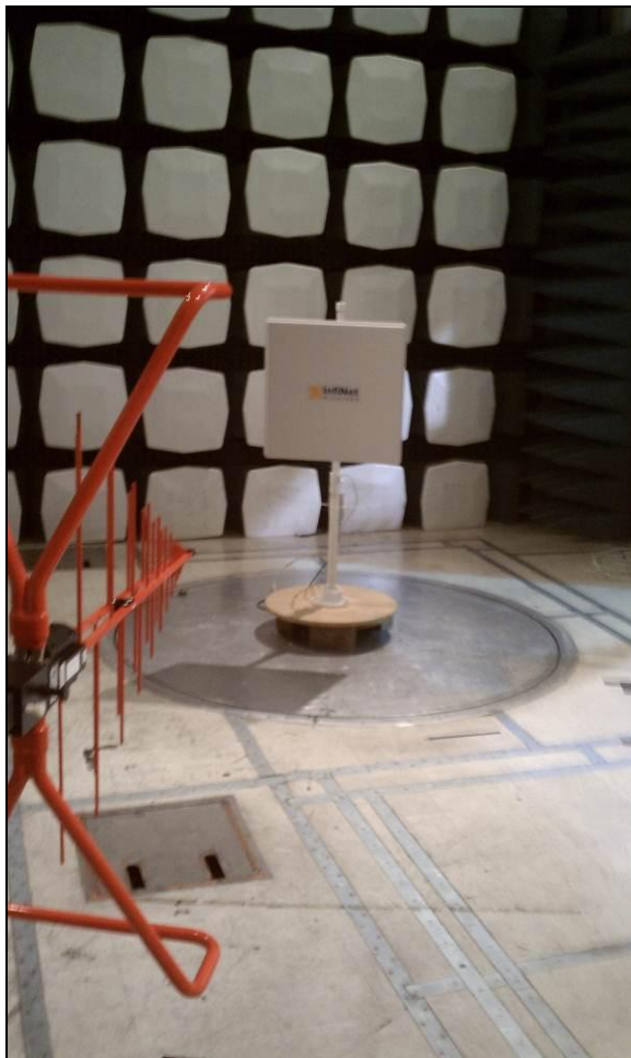
Photograph 3. Radiated Emission, Test Setup
