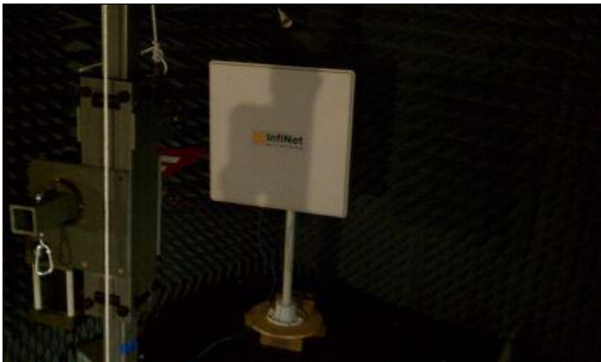
Photograph 5. Radiated Spurious Emissions, Test Setup
