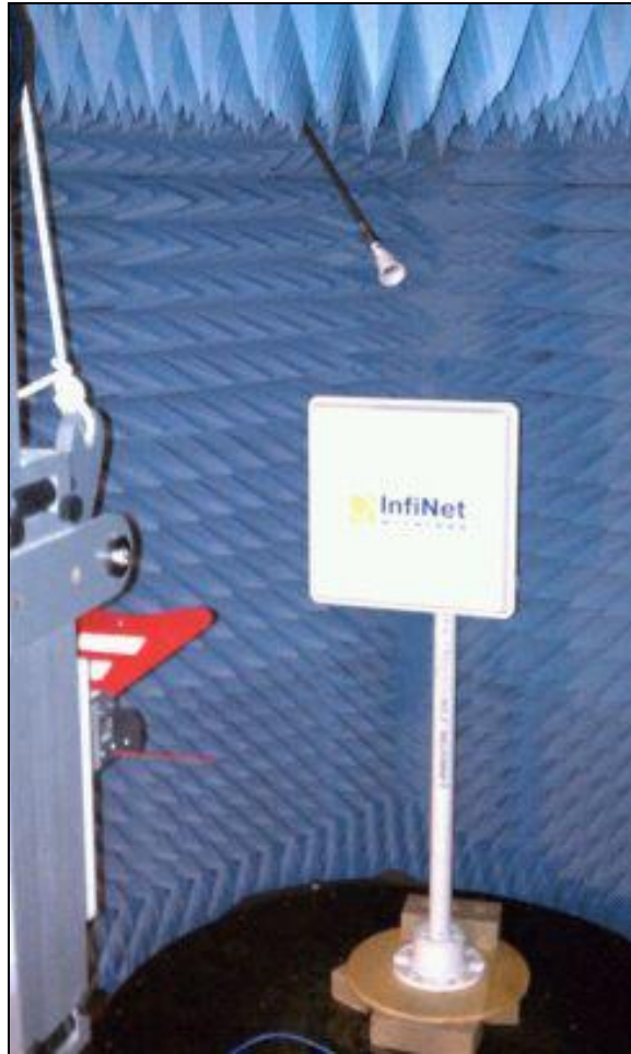
Photograph 5. Radiated Spurious Emissions, Test Setup
