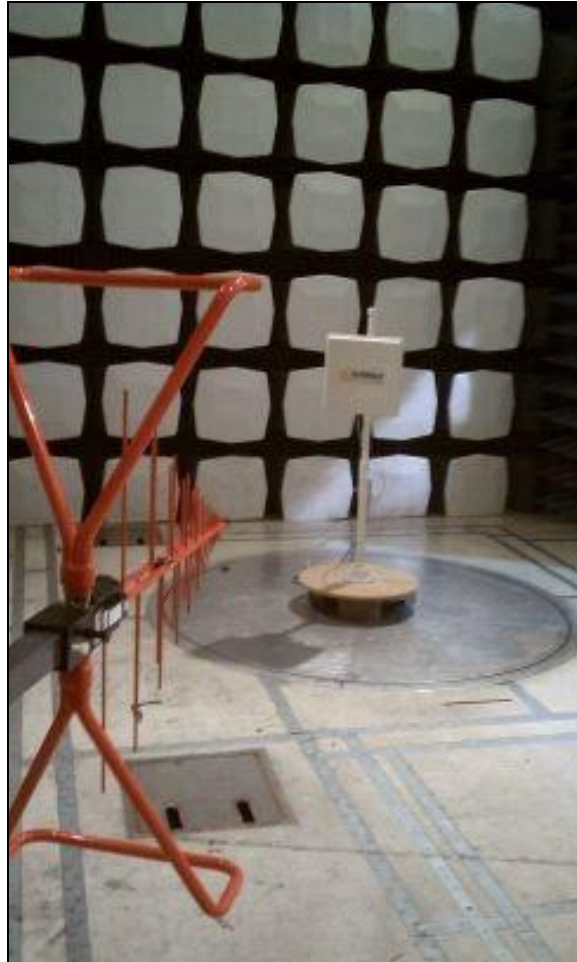
Photograph 2. Conducted Emissions, Test Setup
