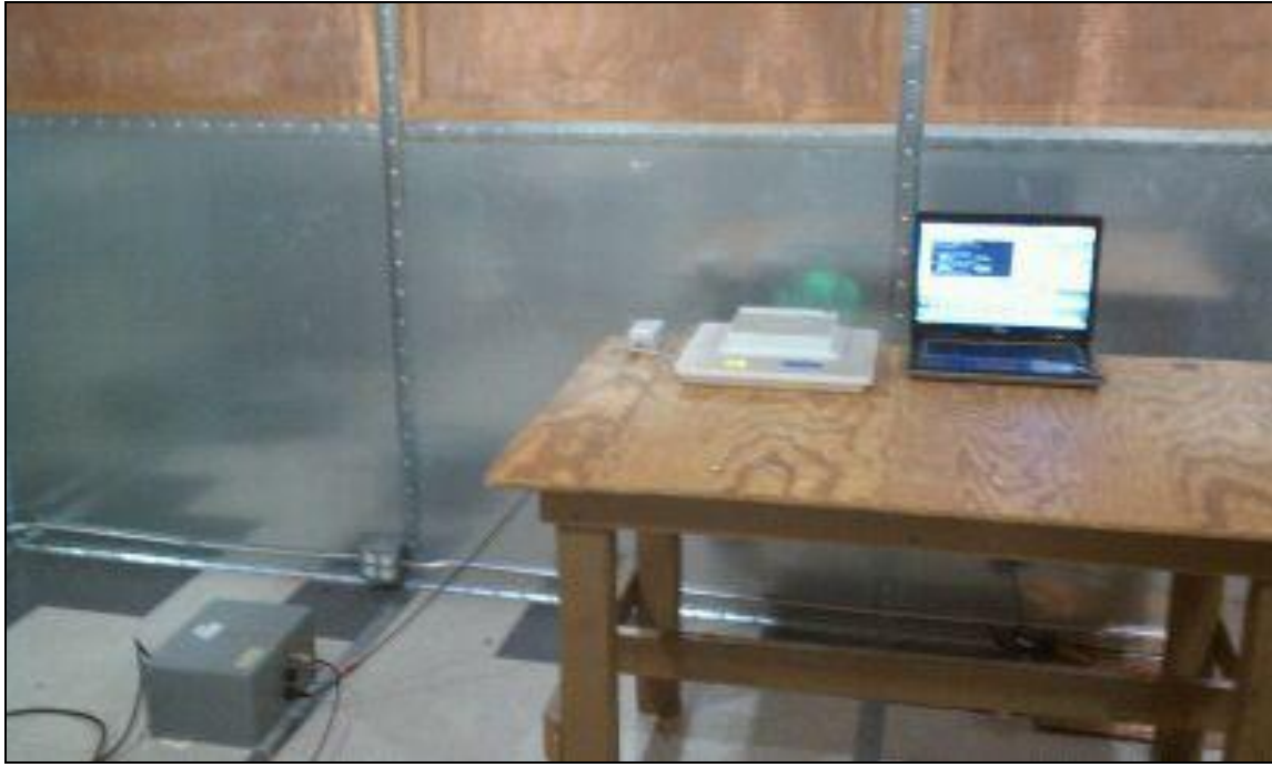
Photograph 4. Conducted Emissions, 15.207(a), Test Setup
