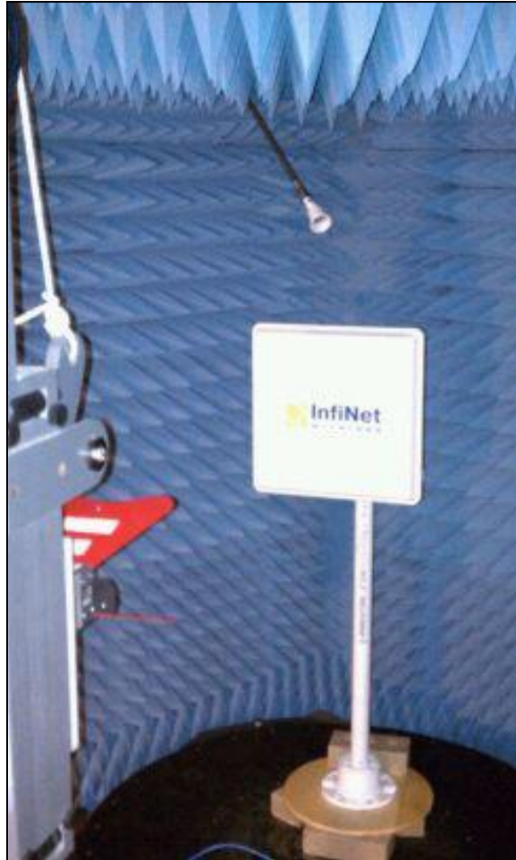
Photograph 3. Radiated Emission, Test Setup
