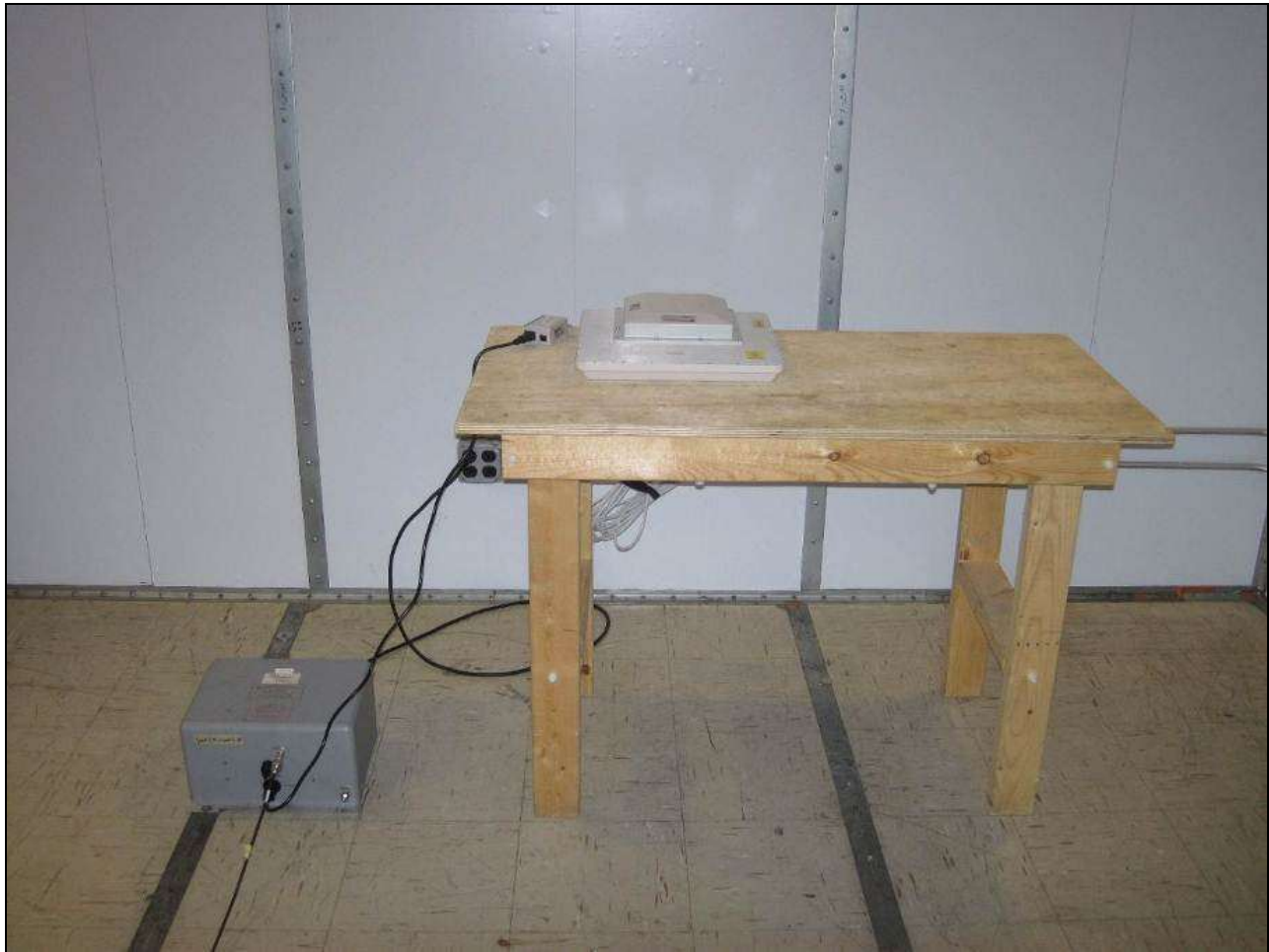
Photograph 2. Conducted Emissions, Test Setup
