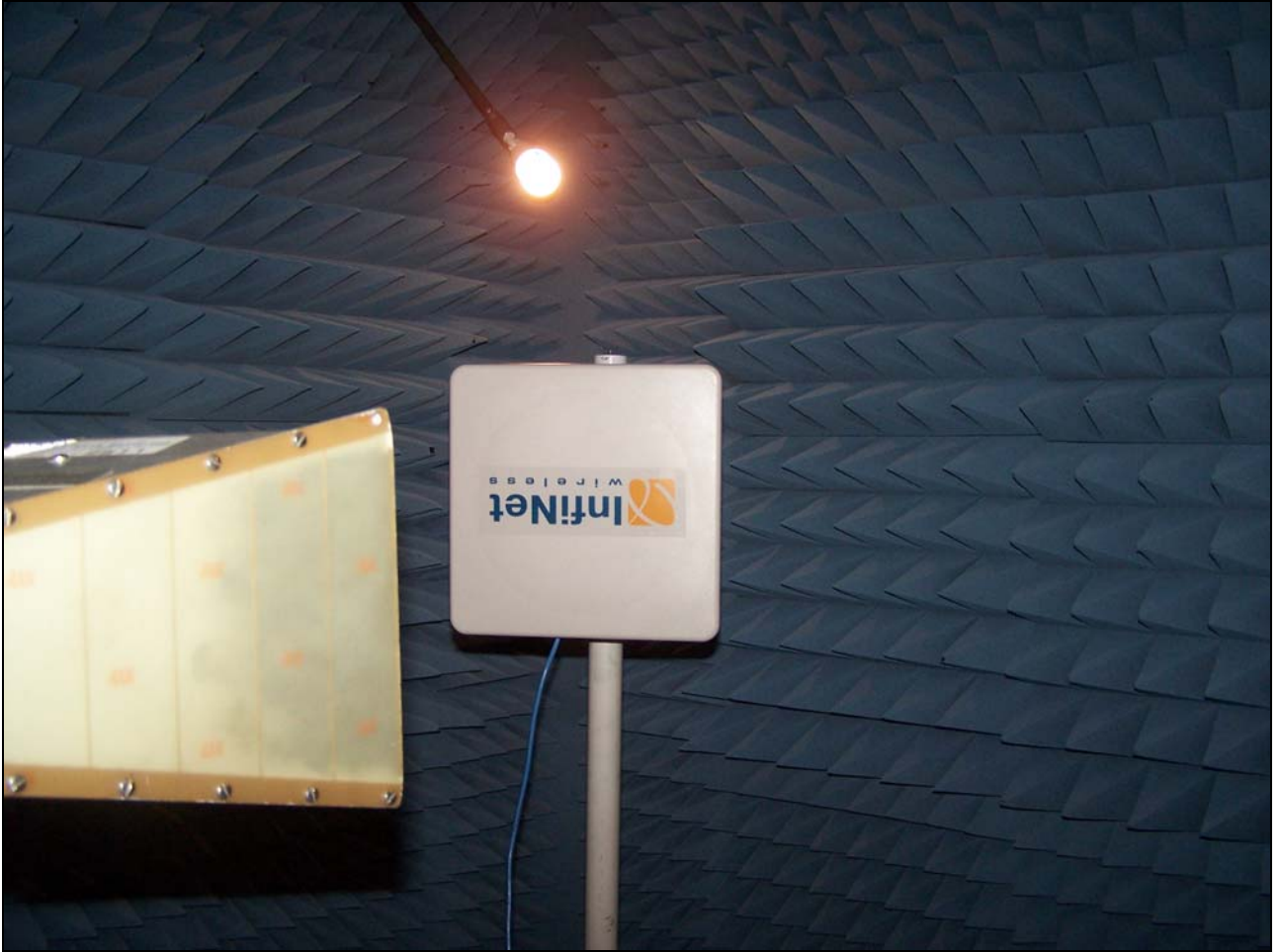
Photograph 4. Radiated Spurious Emissions, Test Setup, Above 1 GHz
