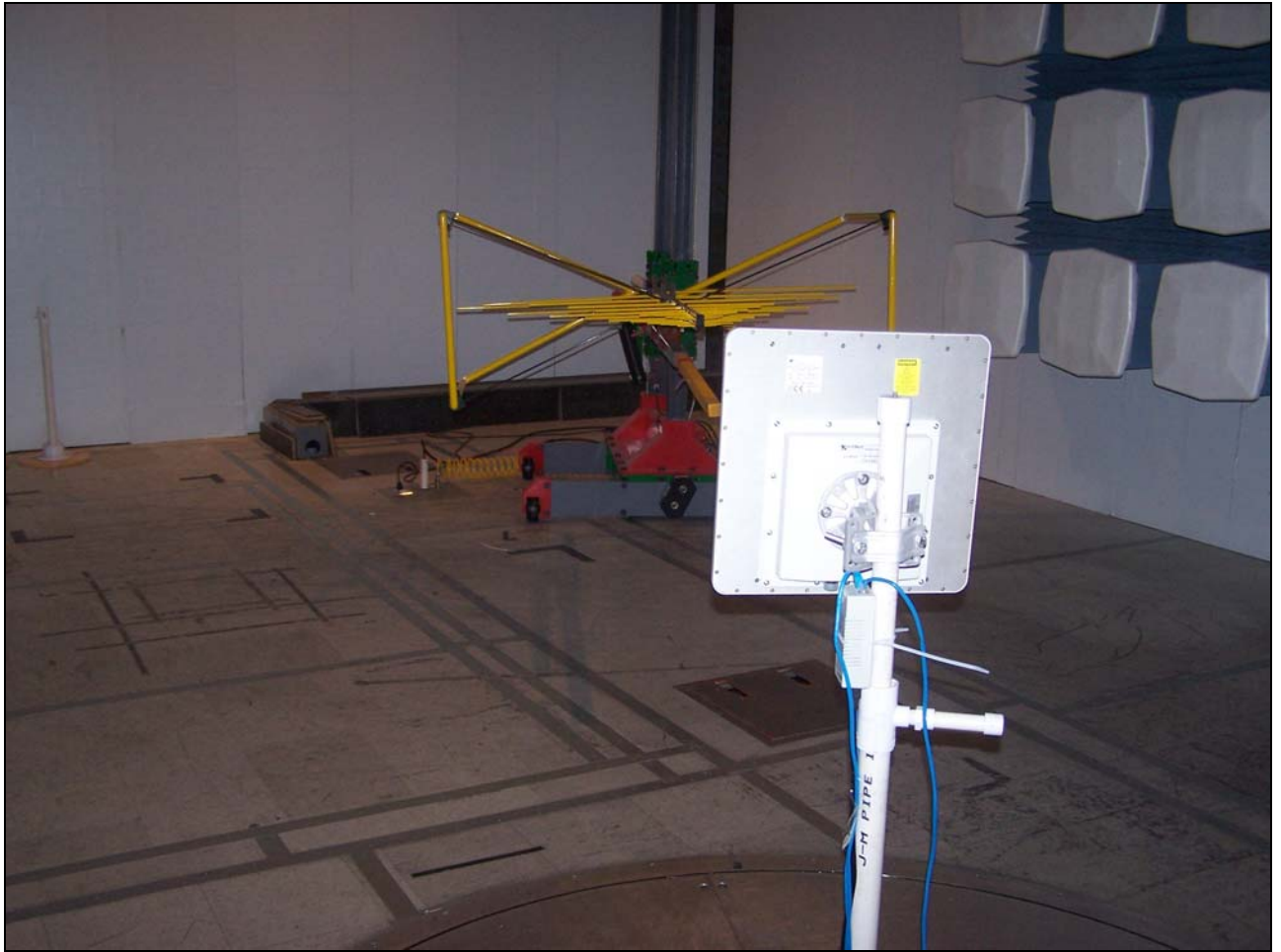
Photograph 3. Radiated Spurious Emissions, Test Setup, Below 1 GHz
