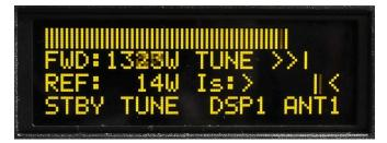
Two of important information is visible – screen current increased, but still is within the allowed limits. Turn LOAD knob slightly in arrows direction to get TUNE indicator between arrows.
