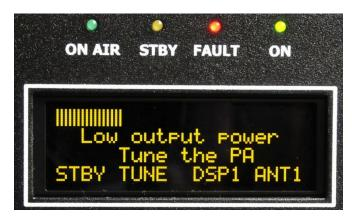
Safety circuit stopped transmitting, fault LED is **ON** (Fault code 4 is saving to the memory).
