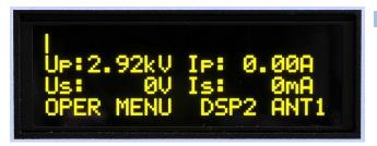
Without RF power the plate voltage is OK.
