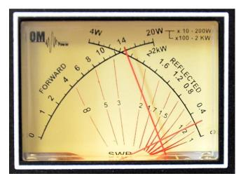
View on the properly tuned PA. Analog wattmeter shows forwarded and reflected power.
