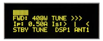
Another example of not optimal result, TUNE indicator must go between both arrows. Use **TUNE** knob **to get maximum output power** and **LOAD** knob **to get indicator between arrows** (in arrows direction).
