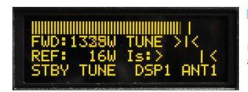
Display indicates **correct tuning** of the Power amplifier.
