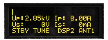
Without RF power the plate voltage is 2.85 kV. Check the heating voltage, too. If it is below 8.5 V, this indicates the need to change AC selector position one step down (for example from 230 to 220 VAC).
