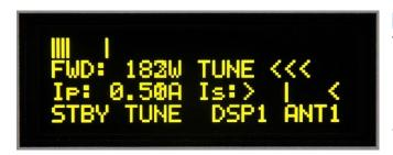
This is not an optimal result, TUNE indicator must go between both arrows. Use **TUNE** knob **to get maximum output power** and LOAD knob **to get indicator between arrows.**
