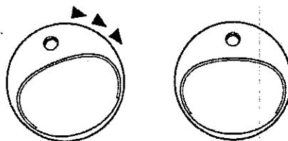
**3** Match the unit to the mounting plate's guide. Rotate the unit clockwise. Your Pathlights are ready for use.
