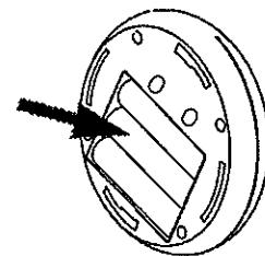
**1** Unscrew the mounting plates from the back of each unit. Fix the mounting plate to the wall using either the enclosed screws or the attached mounting tape. Make sure that the plate is level by referencing the "LEVEL LINE."
