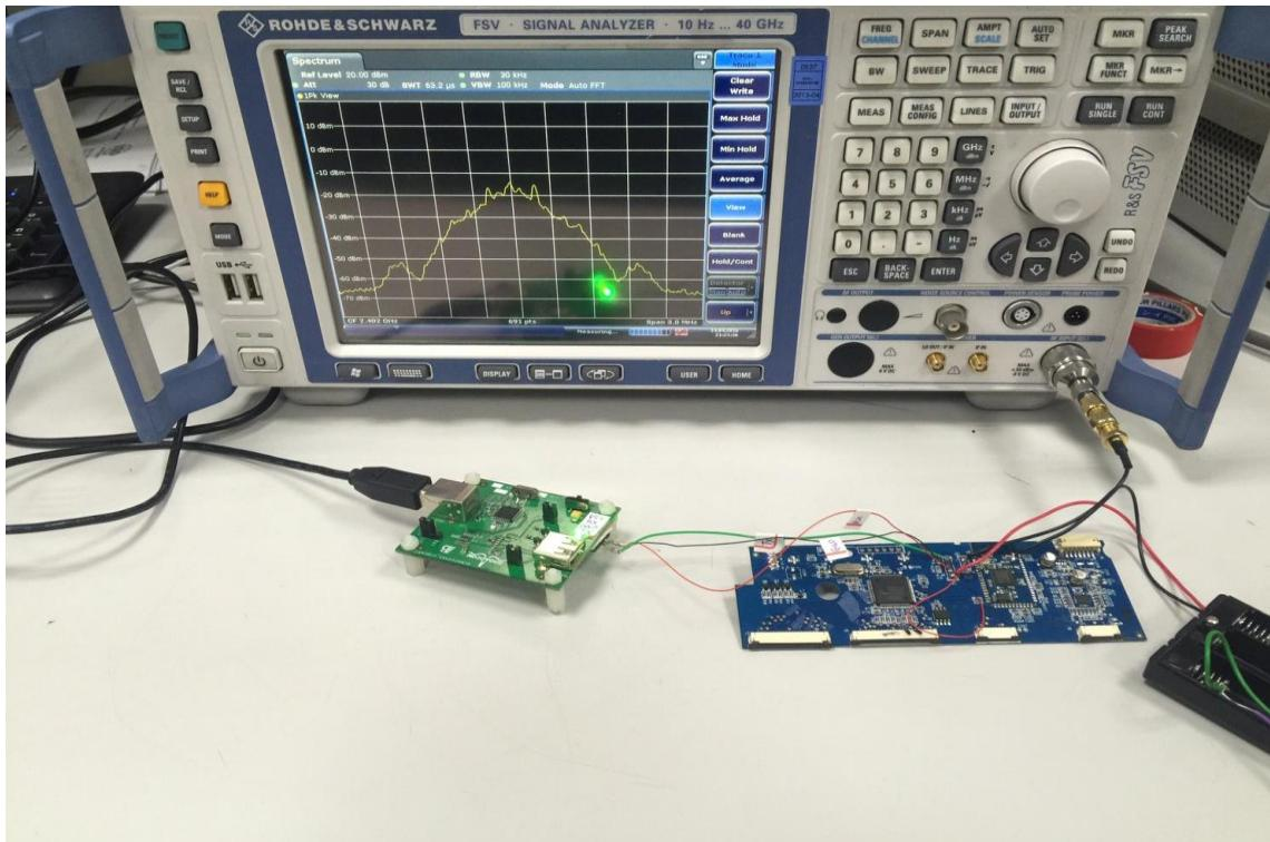
**RADIATED EMISSION SETUP PHOTOS****Below 1GHz**
