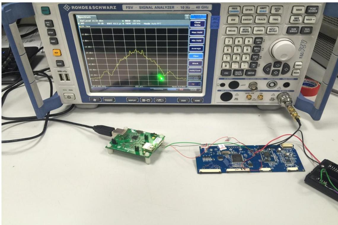
**RADIATED EMISSION SETUP PHOTOS****Below 1GHz**
