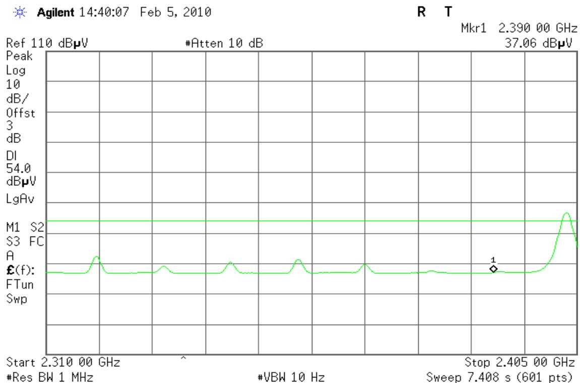
**Detector mode: Peak****Polarity: Horizontal**
