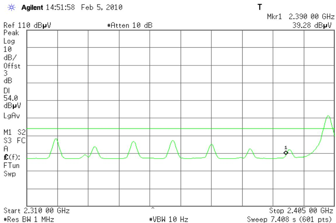
**Band Edges (CH High)****Detector mode: Peak****Polarity: Vertical**
