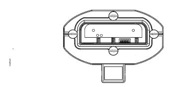
Replace the battery compartment lid and be sure gasket is in place. Use the silicon grease on the gasket to help insure a good water resistant seal. Screw the lid down being sure not to over tighten screws but seating the battery lid and screws firmly and evenly. When screwing down the battery compartment lid, be sure to clear all wires and insure the gasket is in place. The screws should be snug and not over-tightened. The battery compartment lid should not be warped.
