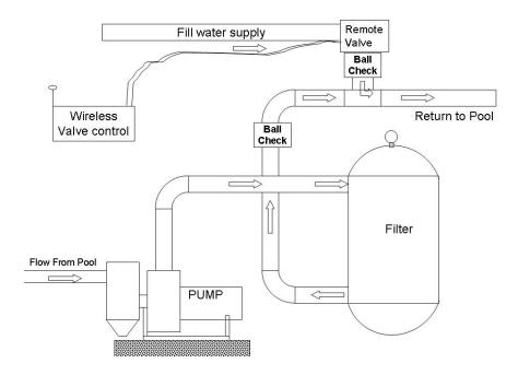
Once you have determined your water supply arrangement and plumbed in the remote valve, you can mount the valve controller where it can receive a strong signal from the Pod sensor. After you mount the Valve controller You will need to run wires from the Valve controller to the solenoid on the valve. The next step is to locate a suitable mounting position based on signal strength for the Valve controller.
