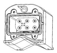
Fill the battery holder with 6 new long life AA batteries, connect the power connector header and insure that lights are flashing and then put the battery cover back on being sure gasket is in place and all wires are tucked in. now is a good time for some silicon grease on the gasket. Once the battery door is secure check again to see that at least the green LED is flashing.
