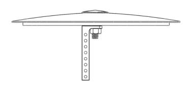
The fully mounted ladder assembly waiting for POD sensor should look like this.
