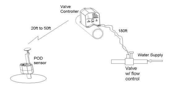
Three major components - Pod Sensor, Valve Controller and remote Water Valve
