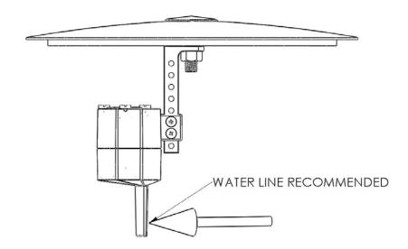
Using the two supplied nylon machine screws and the two small nylon nuts, mount the POD sensor at the correct height in the skimmer onto the mount ladder. Be sure to mount the POD so that the water line is at or near the recommended level. There is no need to be exact but it is a good idea to get as close as possible to the recommended water line when the lid is in place.
