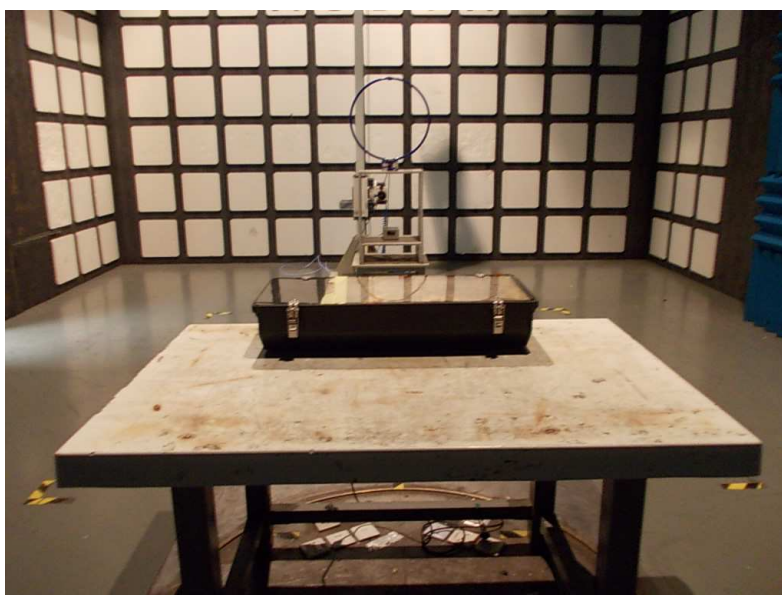
Photograph 2: Set-up for radiated emission
