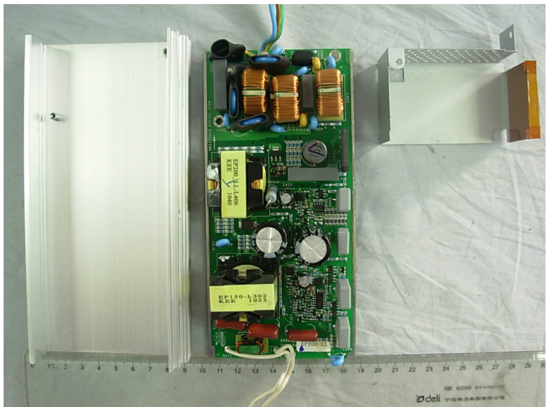
FIGURE 2 ELECTRIC DISCHARGE LAMP CONTROL EQUIPMENT (M/N: SP779#) MAIN BOARD REMOVED
