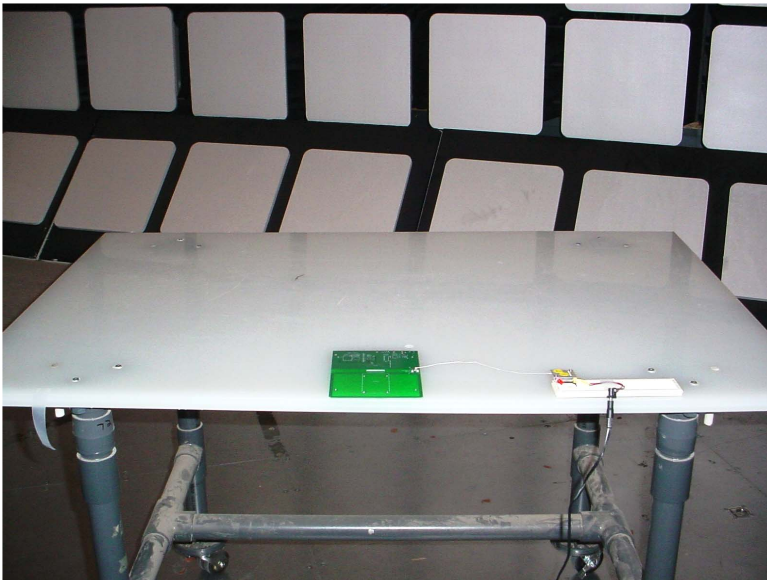
Photo #6: Radiated Emissions, Orthogonal Position #1, Embedded PCB Antenna
