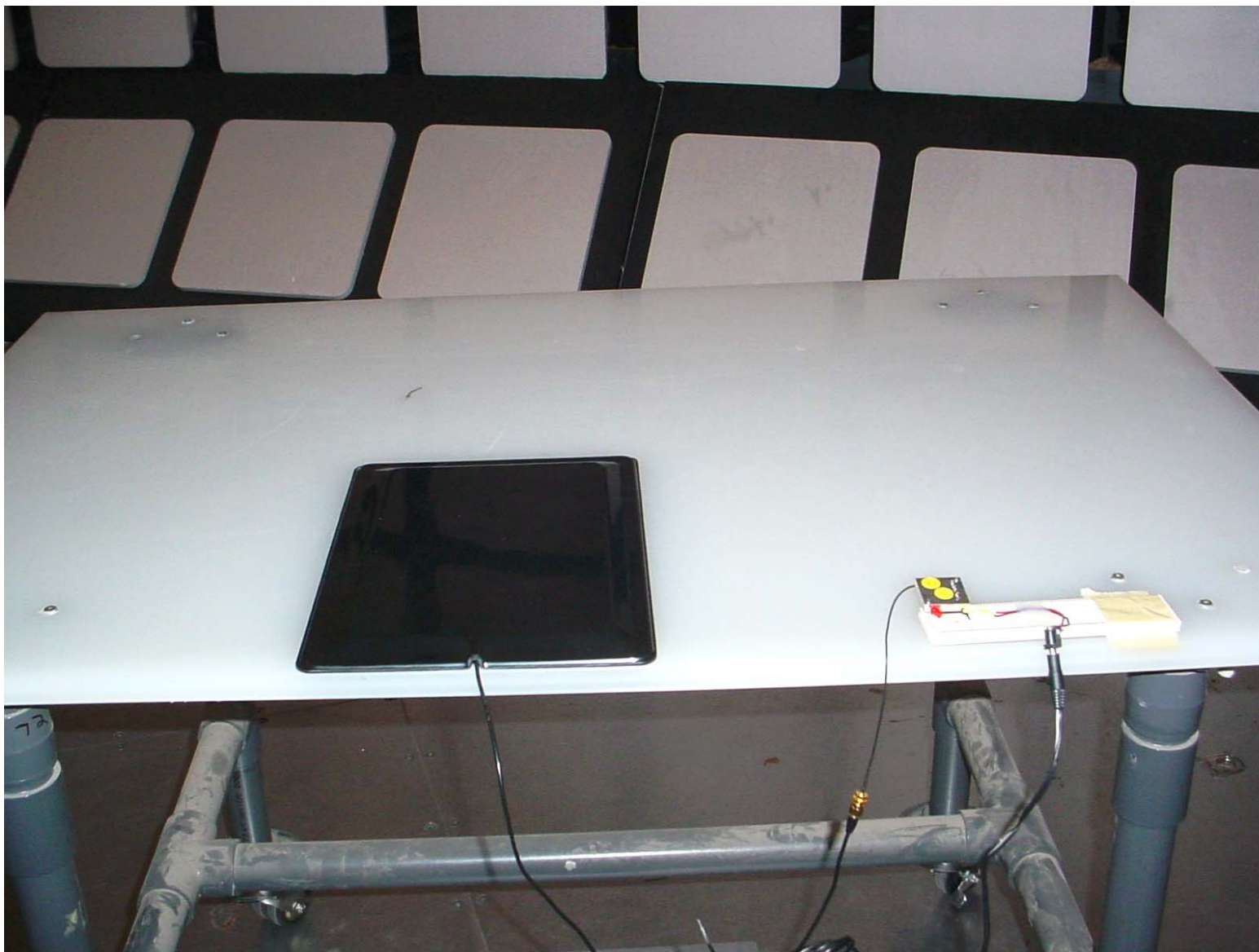
Photo #2: Radiated Emissions, Orthogonal Position #1, Desktop Antenna
