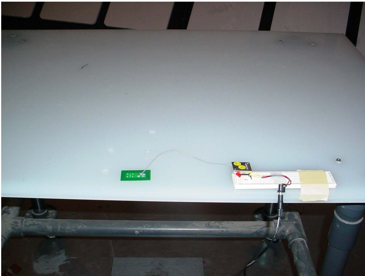
Photo #10: Radiated Emissions, Orthogonal Position #1, Embedded Loop Antenna
