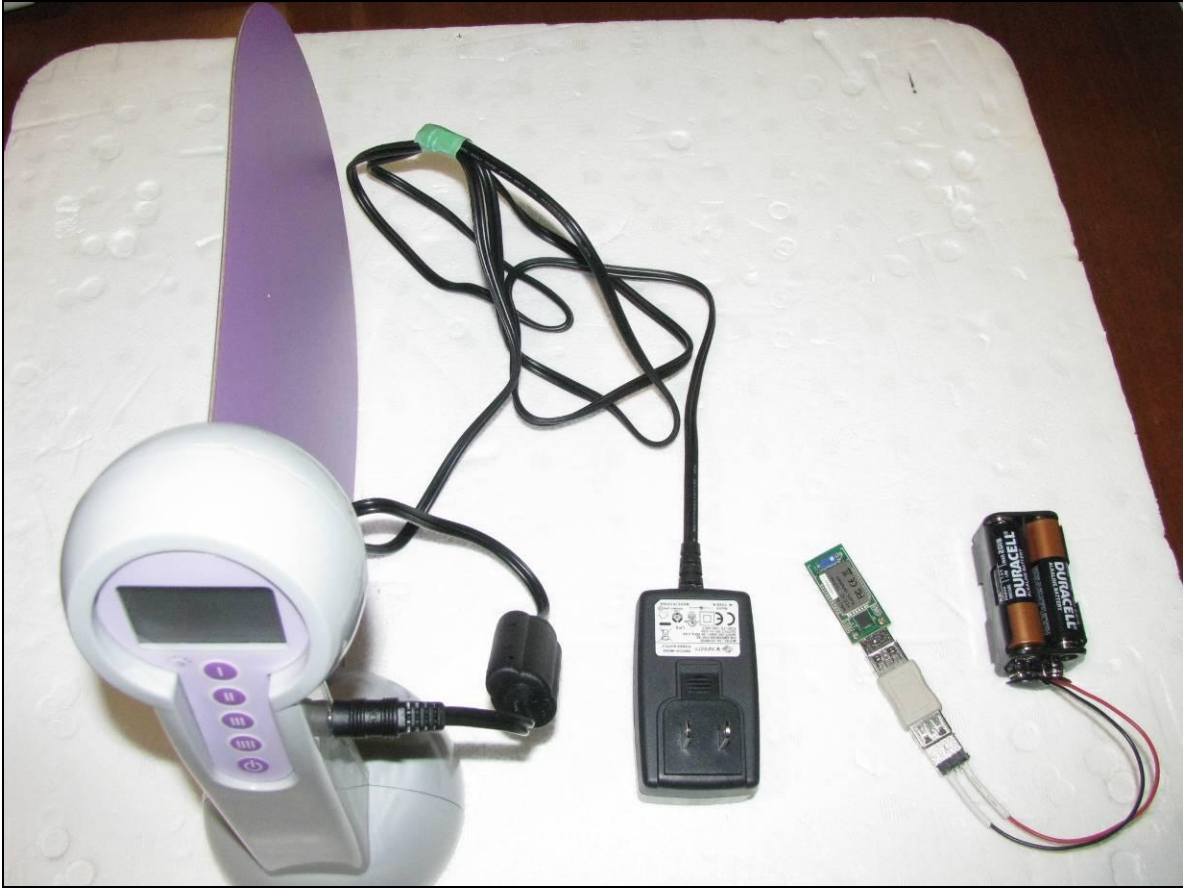
Blade Reader (Scanner) with switch mode power supply/charger and external blue tooth device
