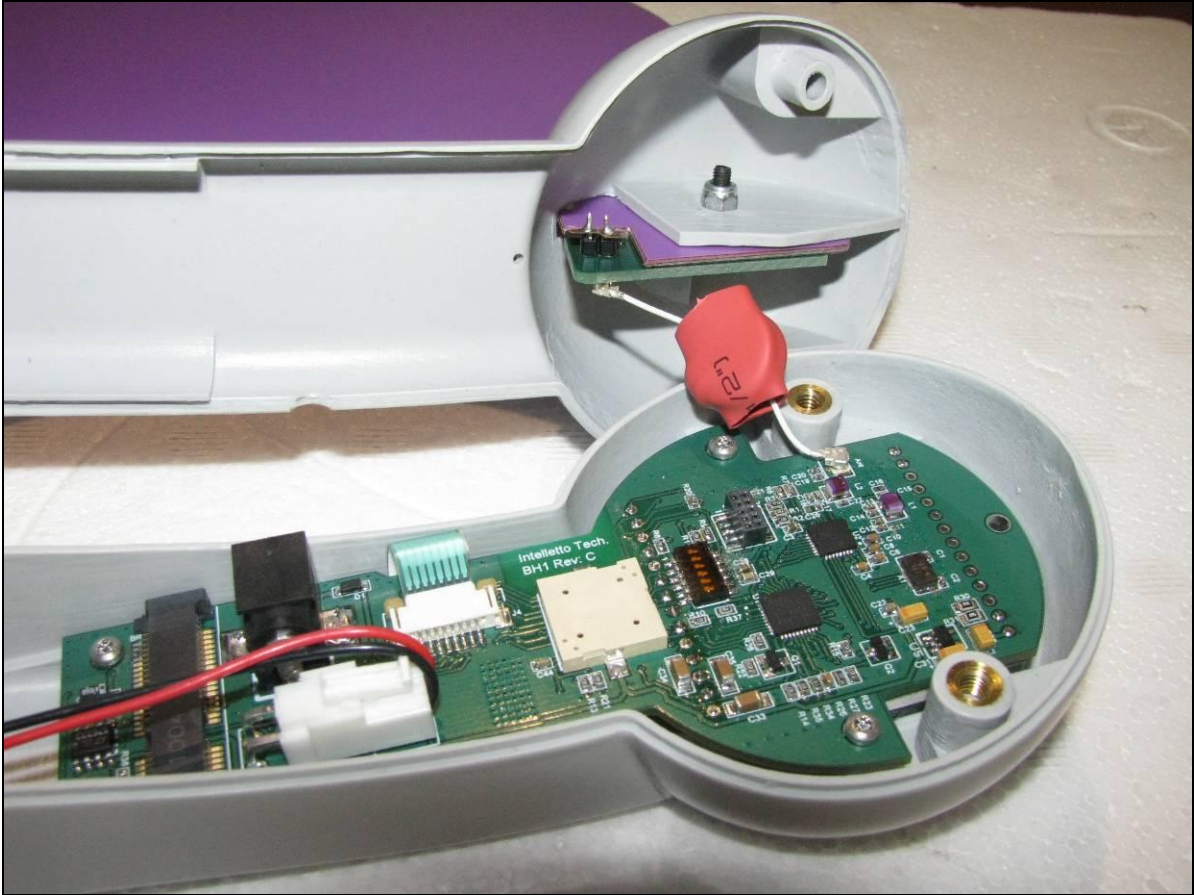
Blade Reader (Scanner) - Internal view2
