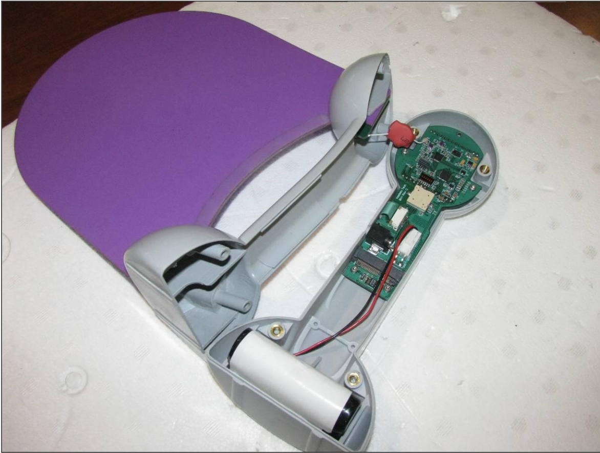
Blade Reader (Scanner) - Internal view1
