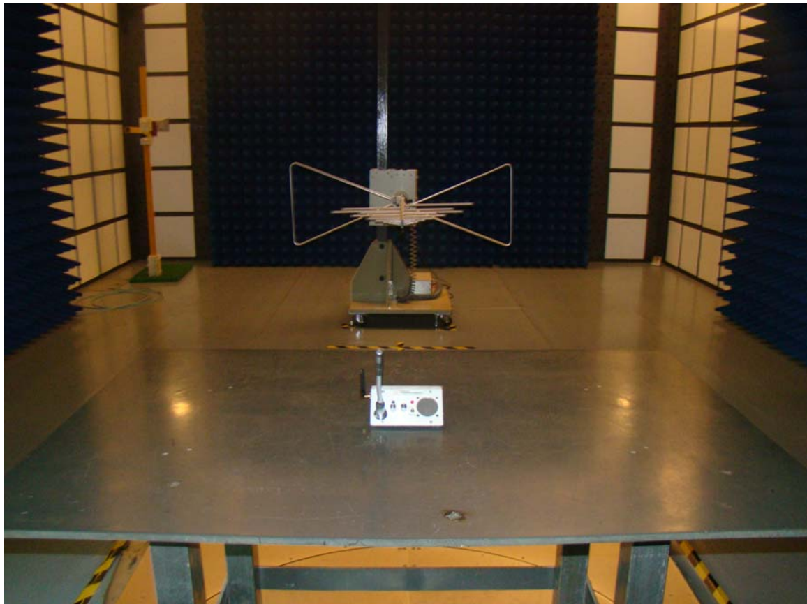
Radiated emissions test < 1GHz
