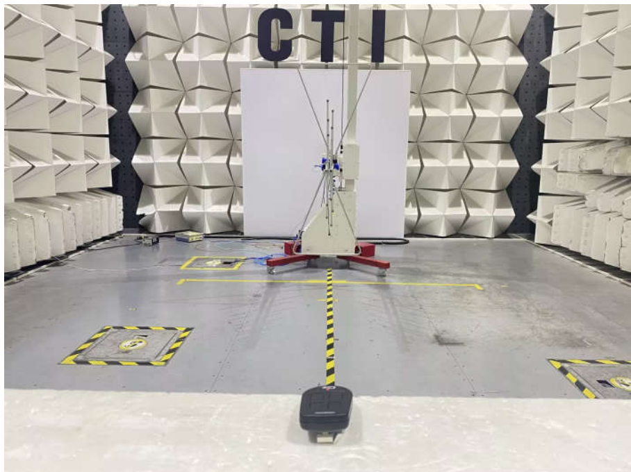
Radiated emission Test Setup-1 (30MHz~1GHz)Close up
