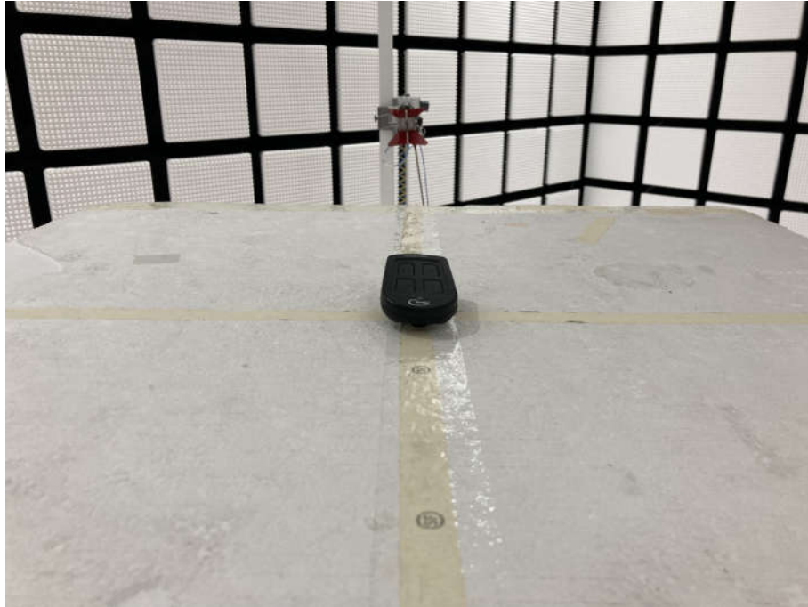
Radiated spurious emission Test Setup-2(Above 1GHz)
