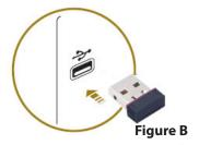
Install the Micro USB receiver (Figure B) into a USB port on the computer or into any of the USB ports on the charging station and wait for the device to Plug and Play. Your Seal Shield™ mouse is designed to use the default drivers on your computer, so no additional software is necessary.
