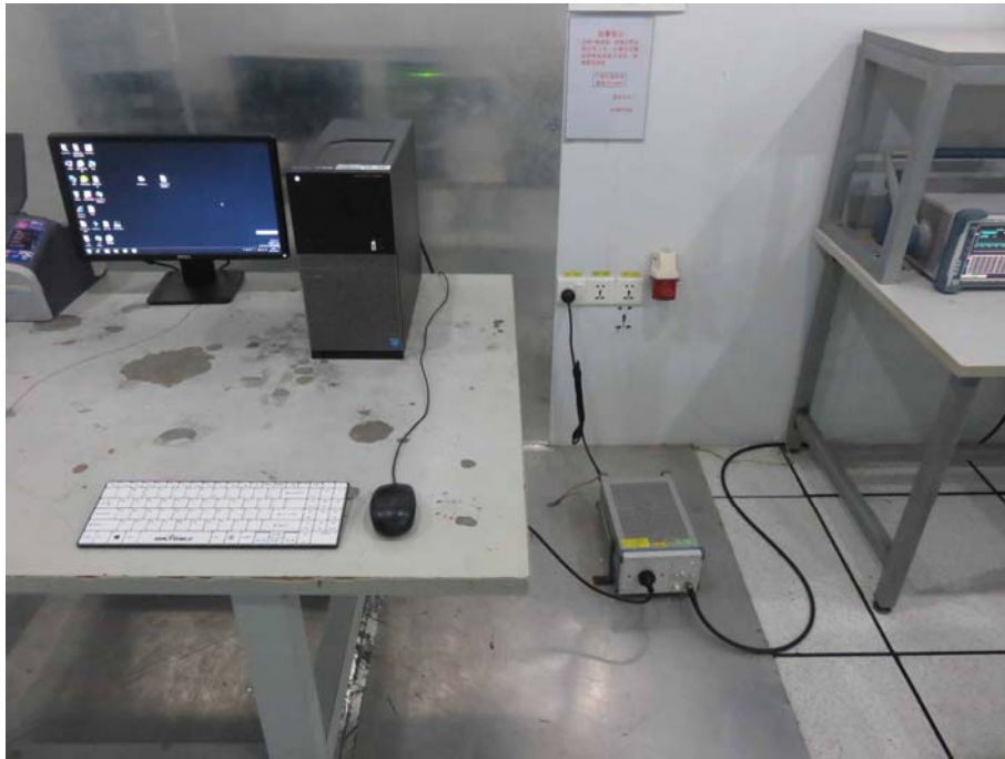
1.1. Photo of Power Line Conducted Emission Test
