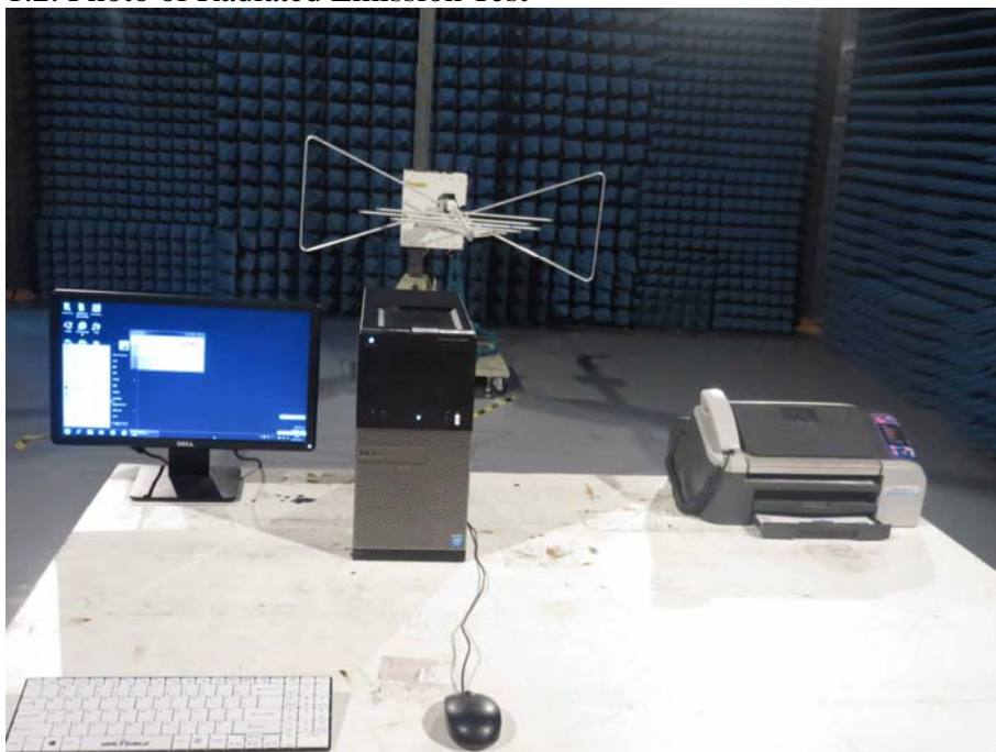
1.2. Photo of Radiated Emission Test
