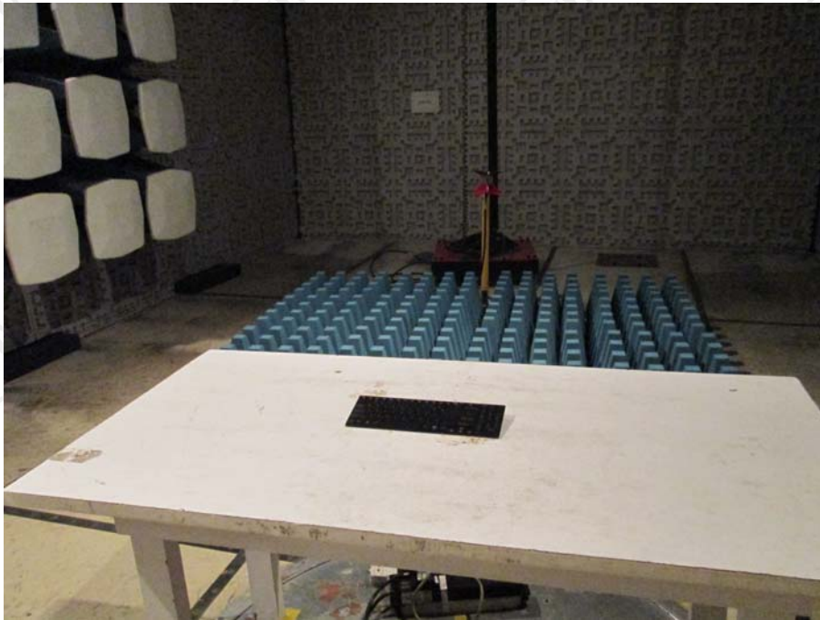
TEST SETUP OF RADIATED EMISSION (above 1GHz)
