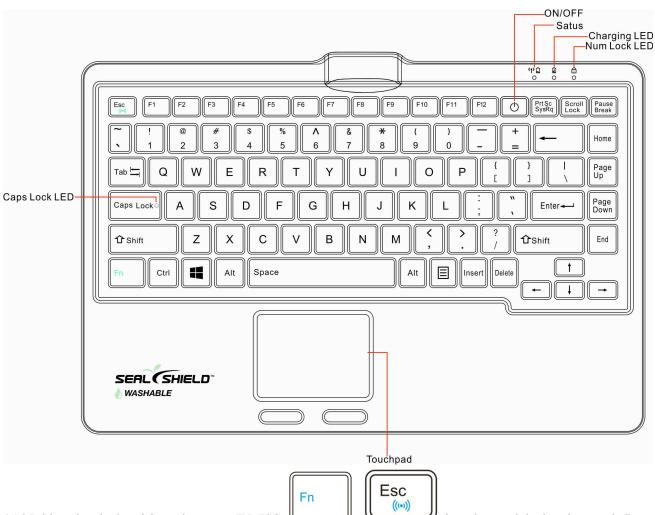
4.1.2.Pairing:when keyboard is on,then press FN+ESC about 3 seconds,keyboard power indicator flashing,now keyboard is entering into pairing status,now can connect with the computer;
