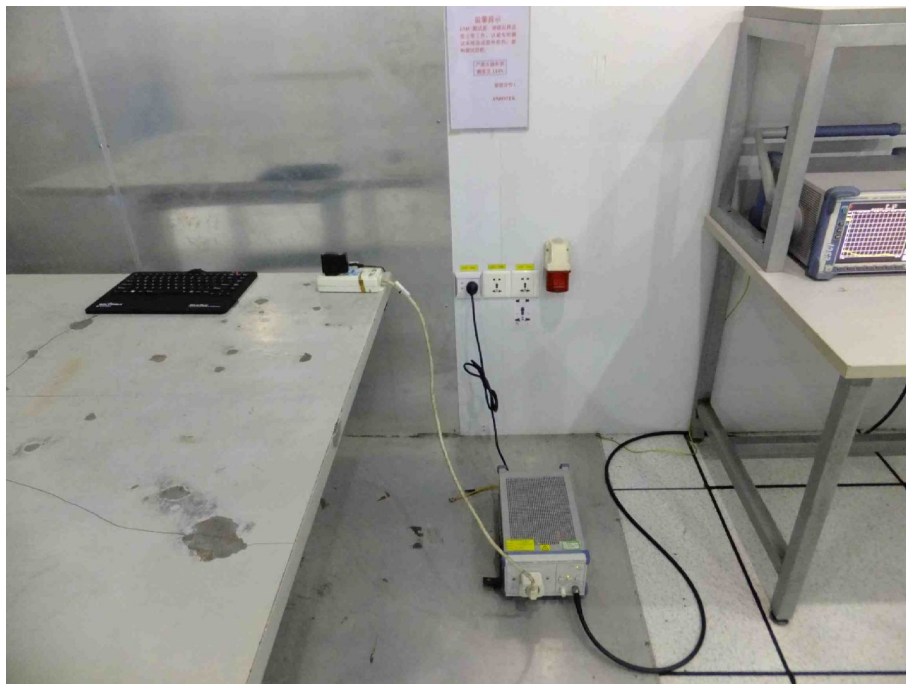
1 Photo of Power Line Conducted Emission Measurement
