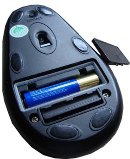
3. Remove the battery door and insert 2 AAA alkaline batteries. Replace the cover and ensure the retainer clamp securely seals the battery door.
