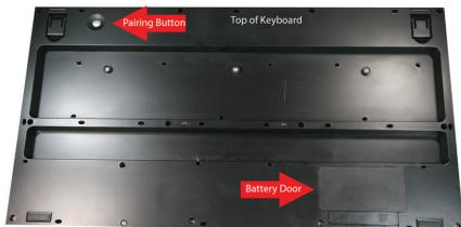
1. Turn the keyboard over and locate the battery door and the pairing button
