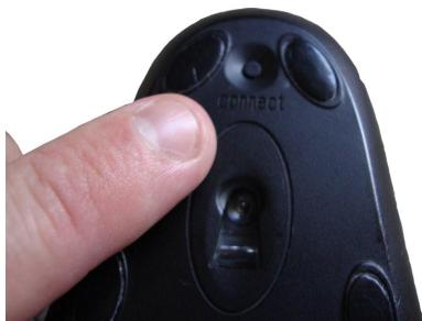
5. Press the Connect button on the bottom of the mouse to pair the mouse to the receiver. The mouse is ready to be used.
