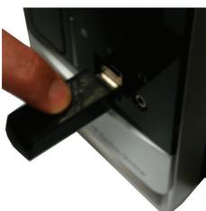
5. Insert the mini receiver into an available USB port and press the white button on the top.
