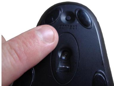
5. Immediately press the Connect button on the bottom of the mouse to pair the mouse to the receiver. The mouse is ready to be used.
