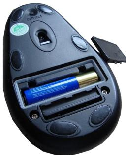
3. Remove the battery door and insert 2 AAA alkaline batteries. Replace the cover and ensure the retainer clamp securely seals the door.
