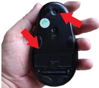
1. Turn the mouse over and locate the battery door and the connect button.
