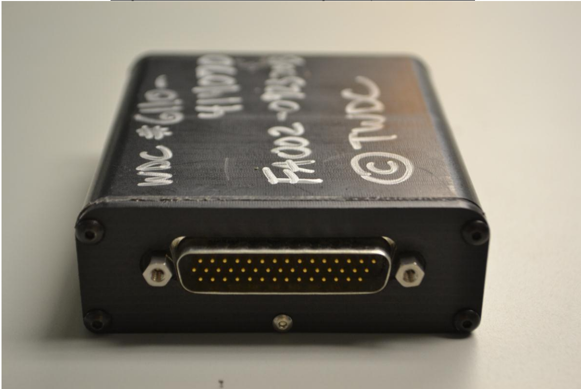
Edge 1 View of the DUT showing battery bus connector
