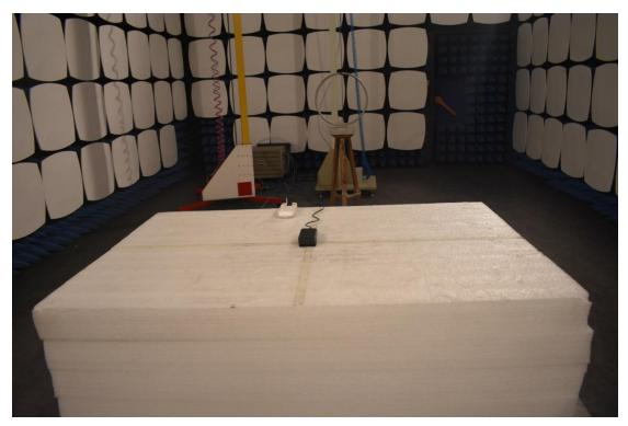
3. Radiated emission (9KHz-30MHz)
