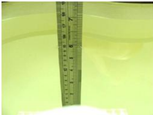
Fig 6.1 Photo of Liquid Height for Head SAR
