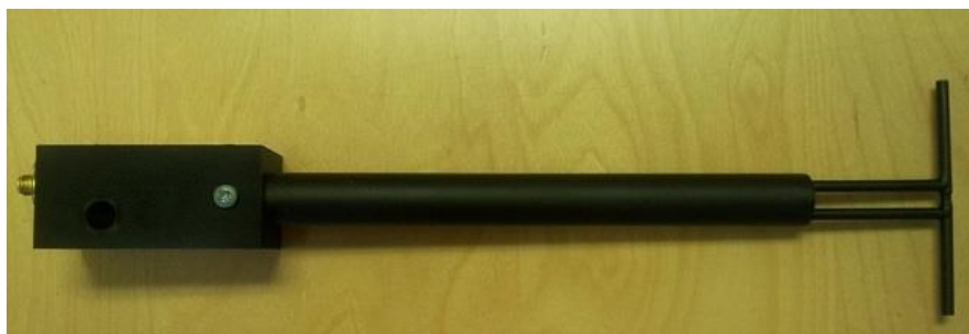
Figure 1 – MVG COMOSAR Validation Dipole
