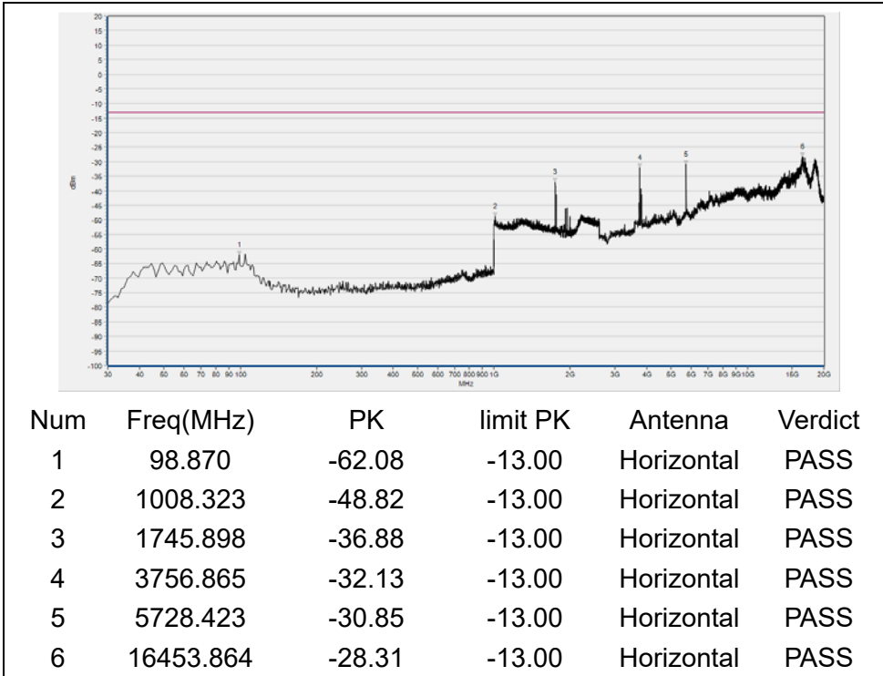
(GPRS 1900MHz, Channel = 810, Horizontal)
