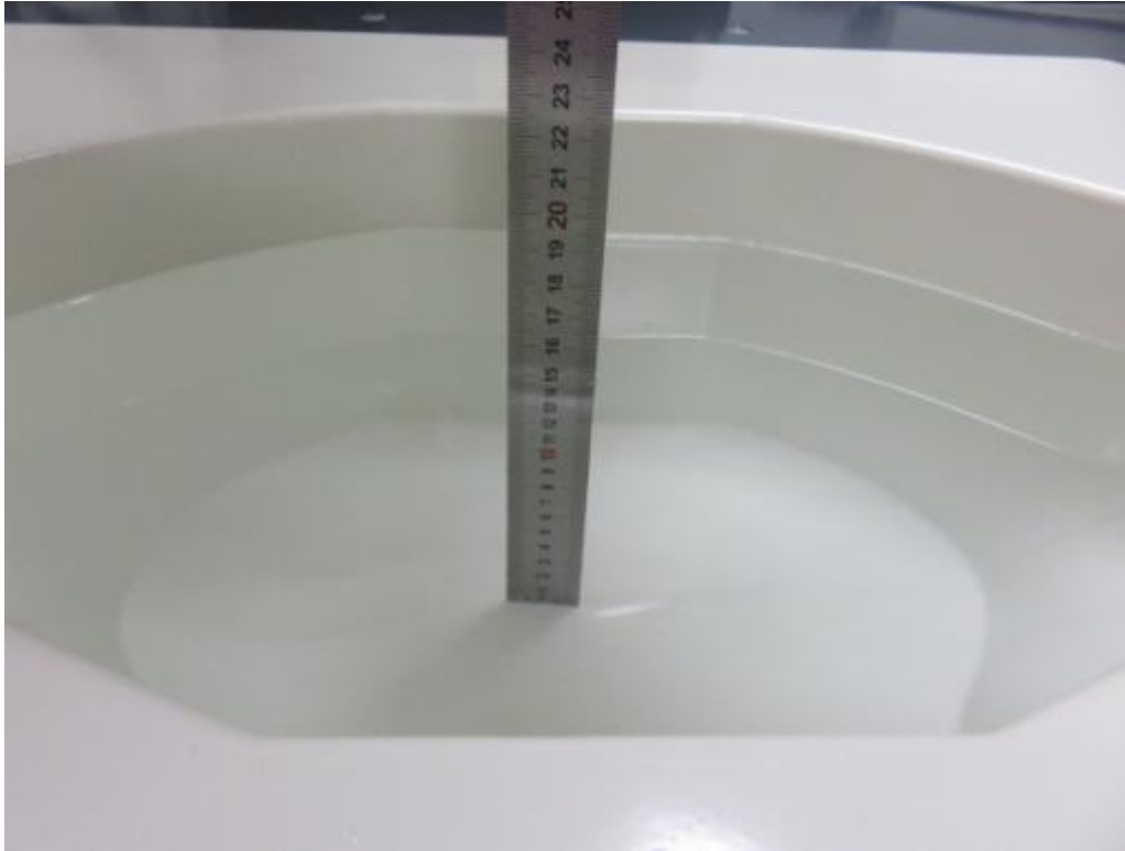
Photograph of the depth in the Body Phantom (835MHz, 16.2cm depth)
