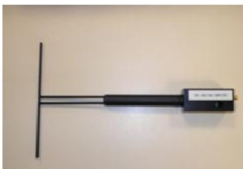
Figure 1 – Satimo COMOSAR Validation Dipole
