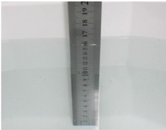
Liquid Height for Head SAR
