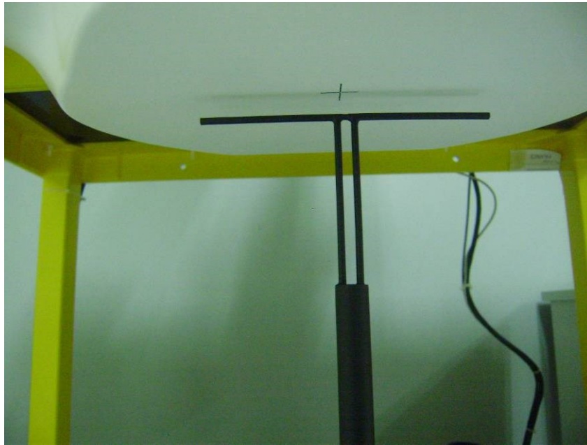
Setup Photo of Dipole Antenna
