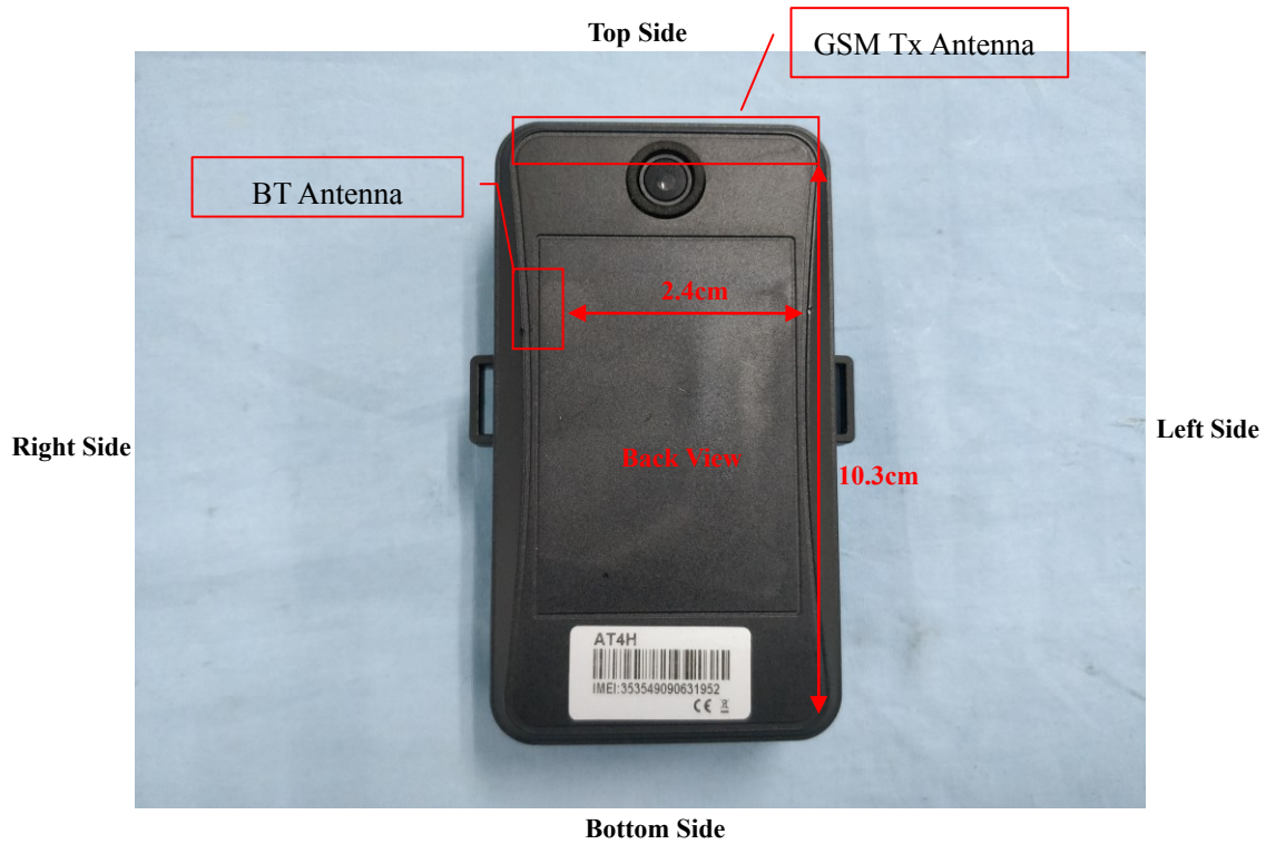
Block Diagram for EUT Antenna Position
