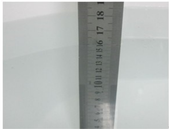
Liquid Height for Body SAR
