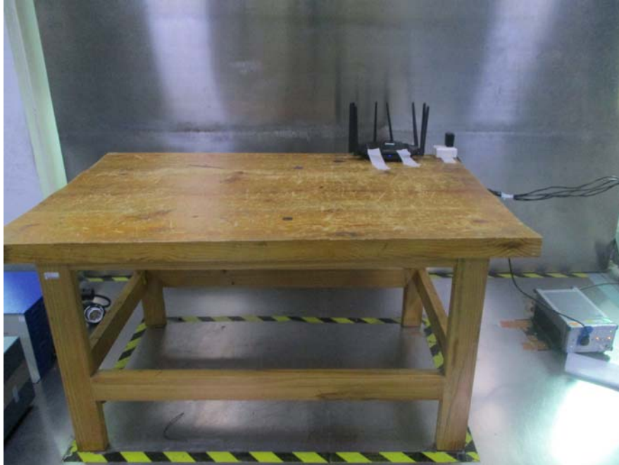
Conducted Emissions – Front View(A7000R)
