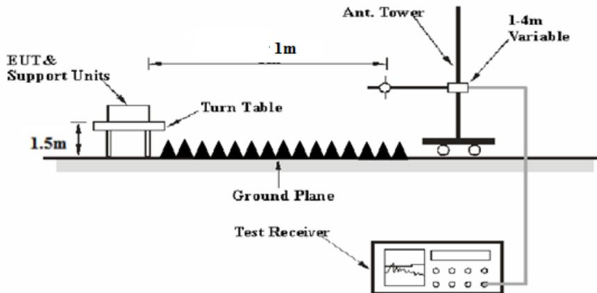
The radiated emission Below 1GHz tests were performed in the 10 meters chamber test site , above 1GHz tests were performed in the 3 meters chamber test site B, using the setup accordance with the ANSI C63.10-2013. The specification used was the FCC 15.209, and FCC 15.407 limits.
