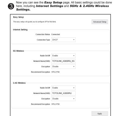
4 of router's WAN port. Choose one **Connection Type** according to your ISP(Internet Service Provider). Connection Status Connected NO. Connection Type Description No configuration, simply connect the WAN port to existing Ethernet port by cable. You're required to enter IP Address, Subnet Mask, Default You're required to enter User Name and Password provided by your ISP. A. DHCP. After choose DHCP, you can go on with the 5GHz & 2.4GHz **Wireless Settings** Connection Type DHCP
