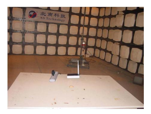
1.4.Set-up for Peak output Power Test
