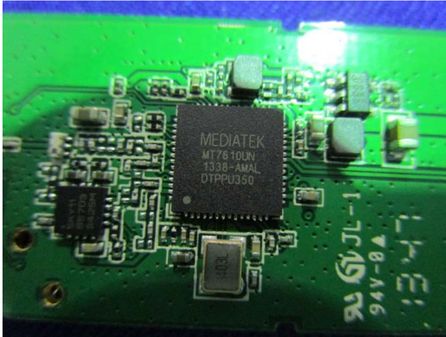
EUT -RF Chip View
