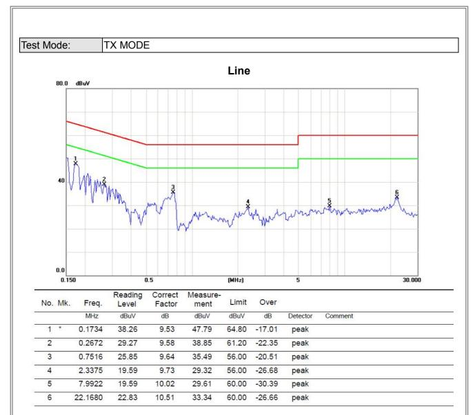
Note: The test result has included the cable loss.
