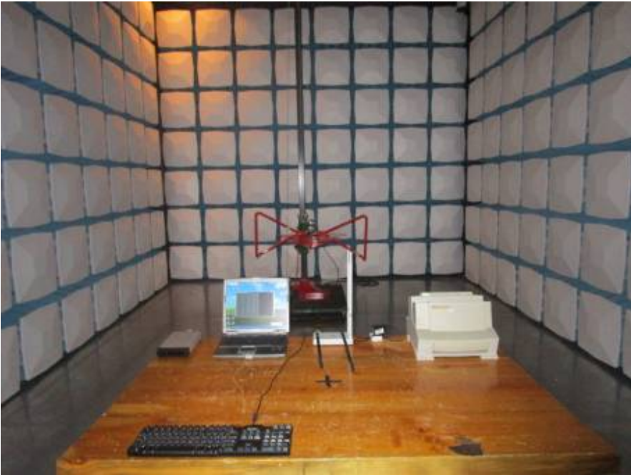
Radiated Emission Below 1GHz -Front View
