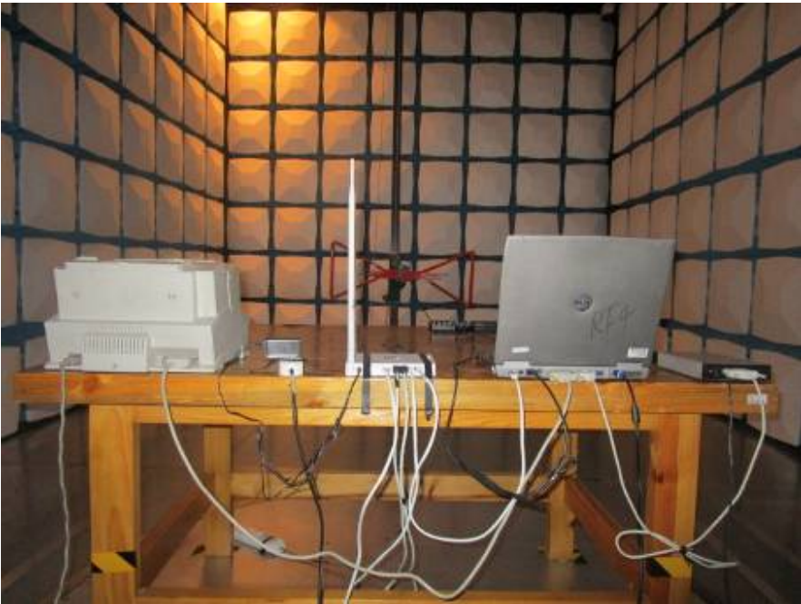
Radiated Emission Below 1GHz - Rear View
