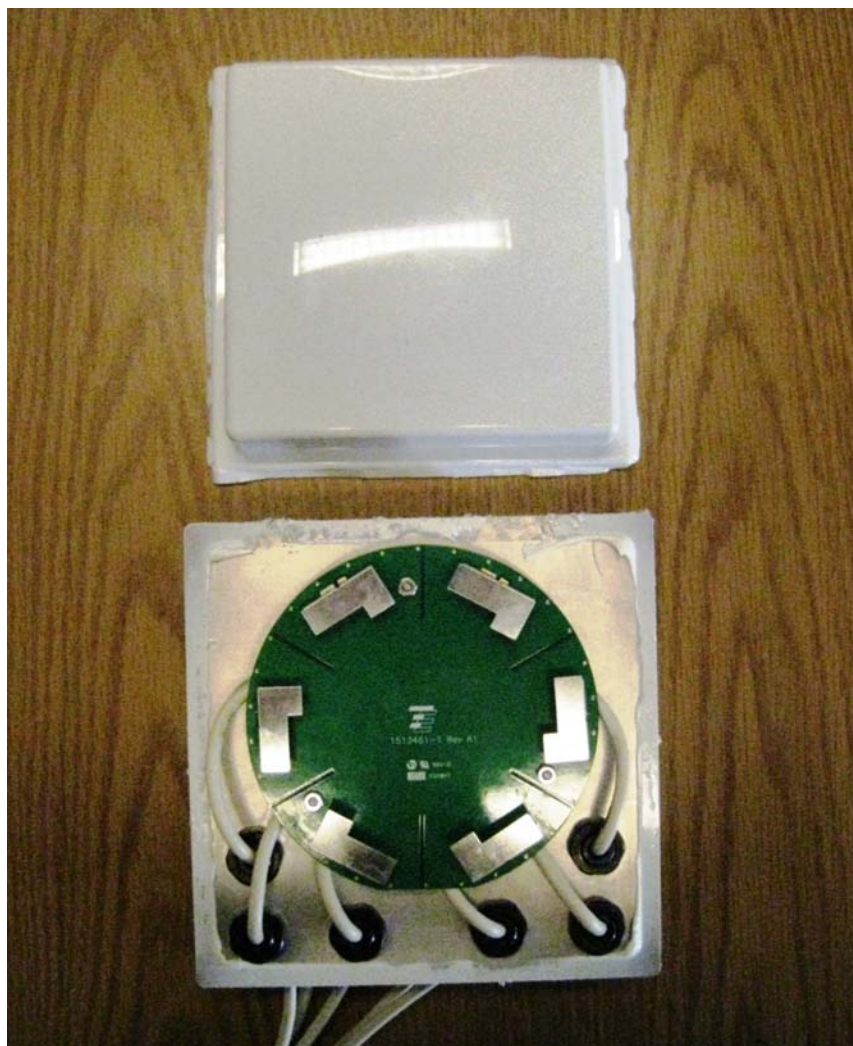
Plastic radome removed showing the same Tyco 1513461-1 Rev A1 antenna as in original filing.
