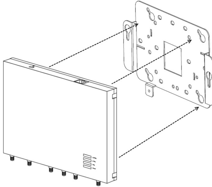
6. Allow the access point to slide down the keyhole slots, making sure the access point mounting tabs are seated at the bottom of the slot.
