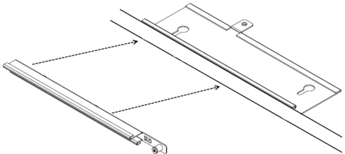
5. Attach the access point to the bracket. Align the access point securing tabs with the keyhole slots in the ceiling grid bracket and carefully slide the access point onto the ceiling grid bracket assembly. If the access point and the bracket assembly are correctly engaged, it should be possible to engage the access points captive thumbscrew into the threaded tab provided on the ceiling grid bracket.
