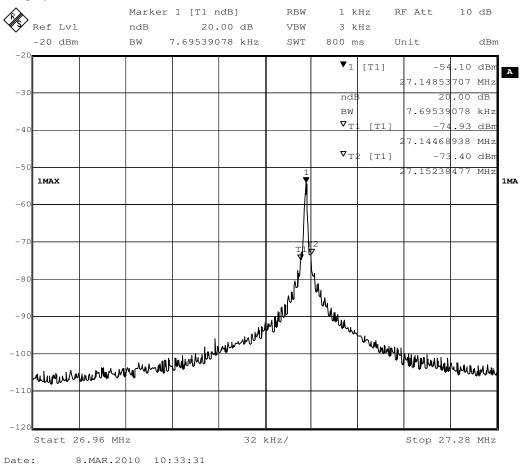
20dB bandwidth lower frequency: 27.14468938MHz 20dB bandwidth upper frequency: 27.15238477MHz
