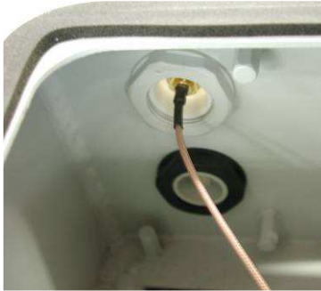
Figure 6 - Antenna plug mounted, internal view
