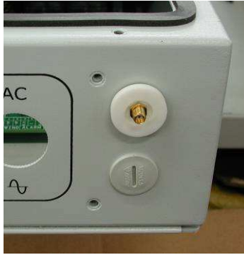
Figure 5 - Antenna plug mounted, external view
