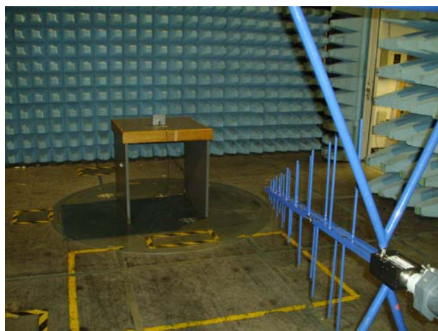
PHOTO 3 – SET-UP FOR EMISSION RADIATED TEST
