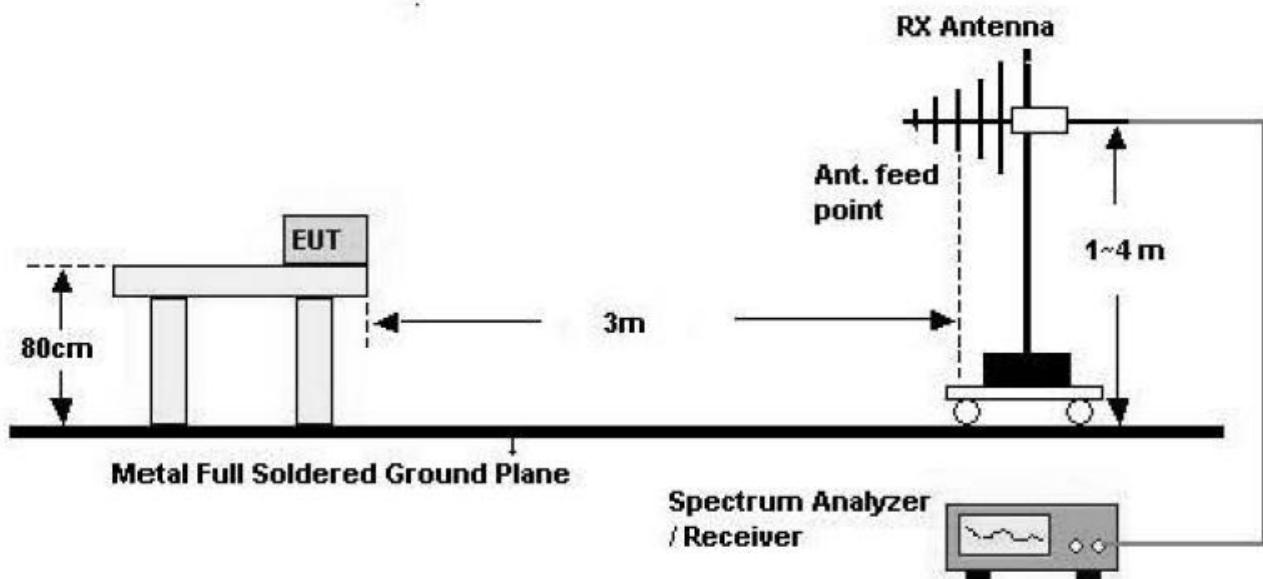
**Above 1 GHz**
