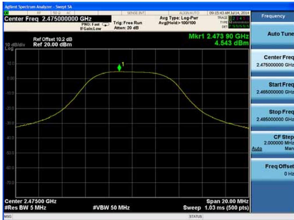
**RESULT PLOTS-Average****Conducted Output Power (Low-CH)**
