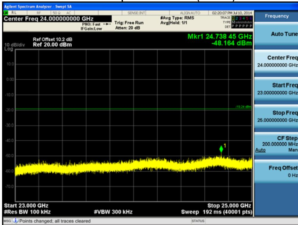
**8.6 RAATED MEASUREMENT.****8.6.1 RAATED SPURIOUS EMISSIONS.****Test Requirements and limit, §15.205, §15.209**
