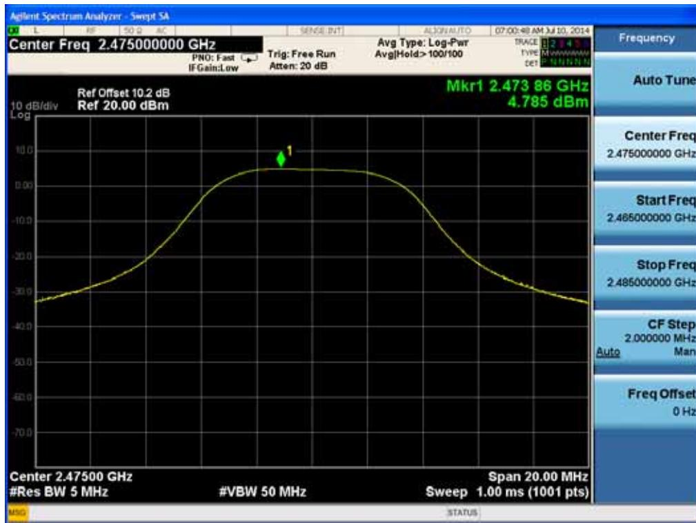
**RESULT PLOTS-Average****Conducted Output Power (Low-CH)**
