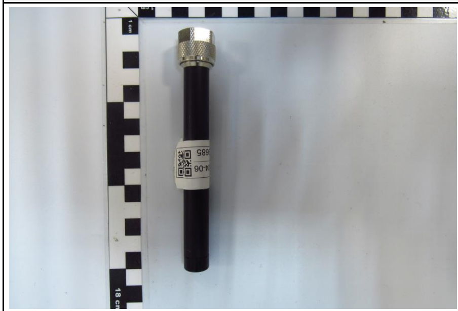
Ancillary equipment: Antenna F9915KW
