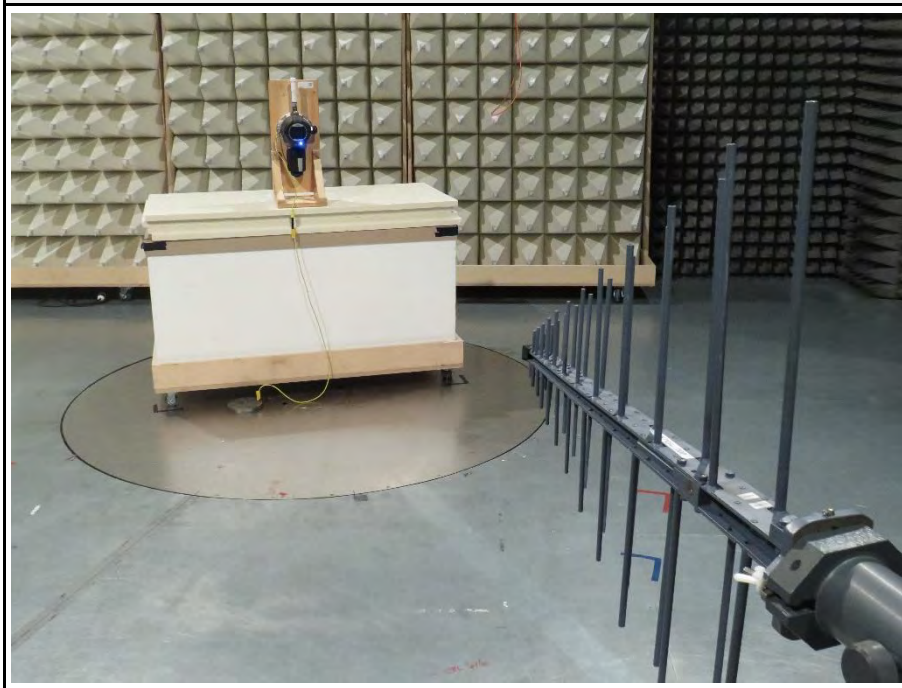
EUT 1 test setup 200 - 1000MHz vertical
