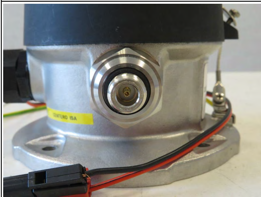
EUT 2 Top antenna connection
