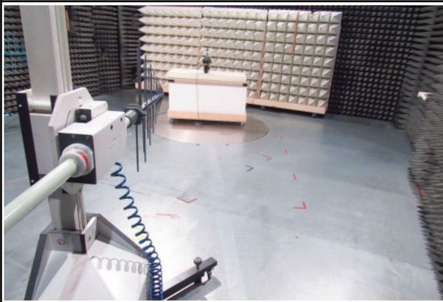
Setup for measurements below 1 GHz
